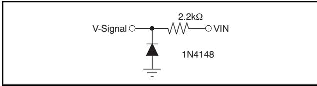
Figure 42. Enhanced Protection Against Negative Overload of  $V_{IN}$
