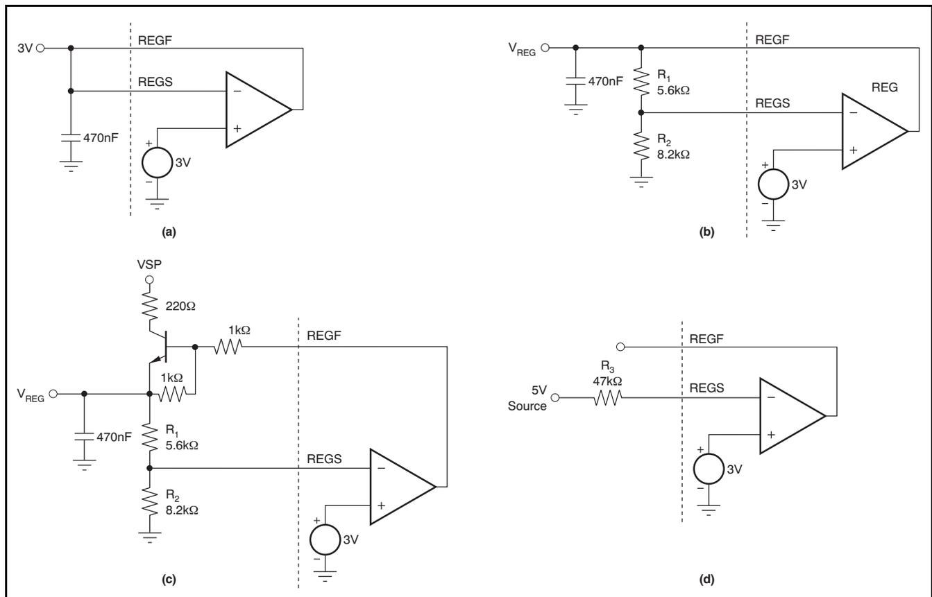
**Figure 45. Basic Connections of the Voltage Regulator**
