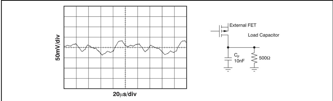
Figure 40. Output with  $10\text{nF}$  Parallel to  $500\Omega$
