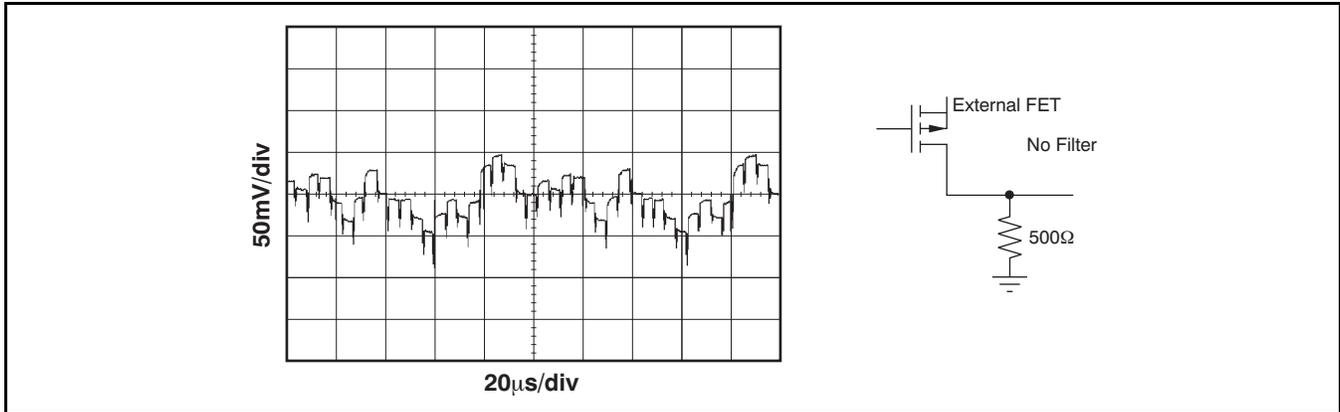
Figure 39. Output Noise without Filter into  $500\Omega$
