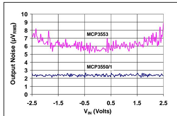
**FIGURE 2-6:** Output Noise vs. Input Voltage ( $V_{DD} = 2.7\text{V}$ ).
