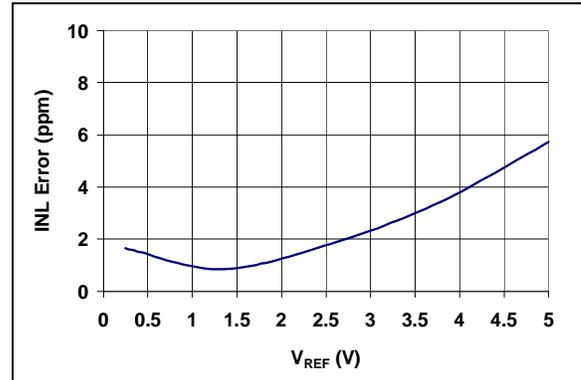
**FIGURE 2-4:** Maximum INL Error vs.  $V_{REF}$ .
