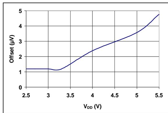
**FIGURE 2-11:** Offset Error vs  $V_{DD}$  ( $V_{CM} = 0\text{V}$ ).
