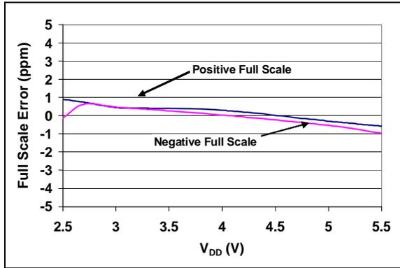
**FIGURE 2-13:** Full Scale Error vs.  $V_{DD}$ .
