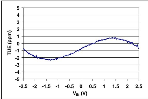
**FIGURE 2-19:** Total Unadjusted Error (TUE) vs. Input Voltage.
