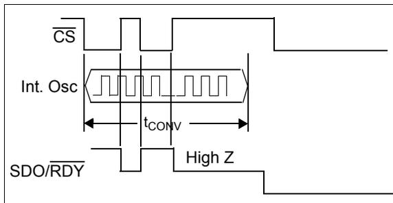
**FIGURE 5-4:** RDY Functionality in Single Conversion Mode.
