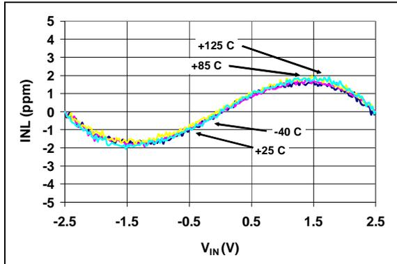
**FIGURE 2-1:** INL Error vs. Input Voltage ( $V_{DD} = 2.7\text{V}$ ).
