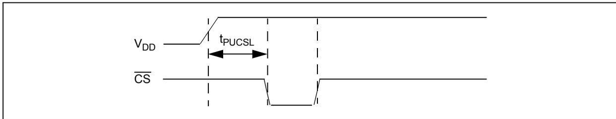
**FIGURE 1-2:** Power-Up Timing.
