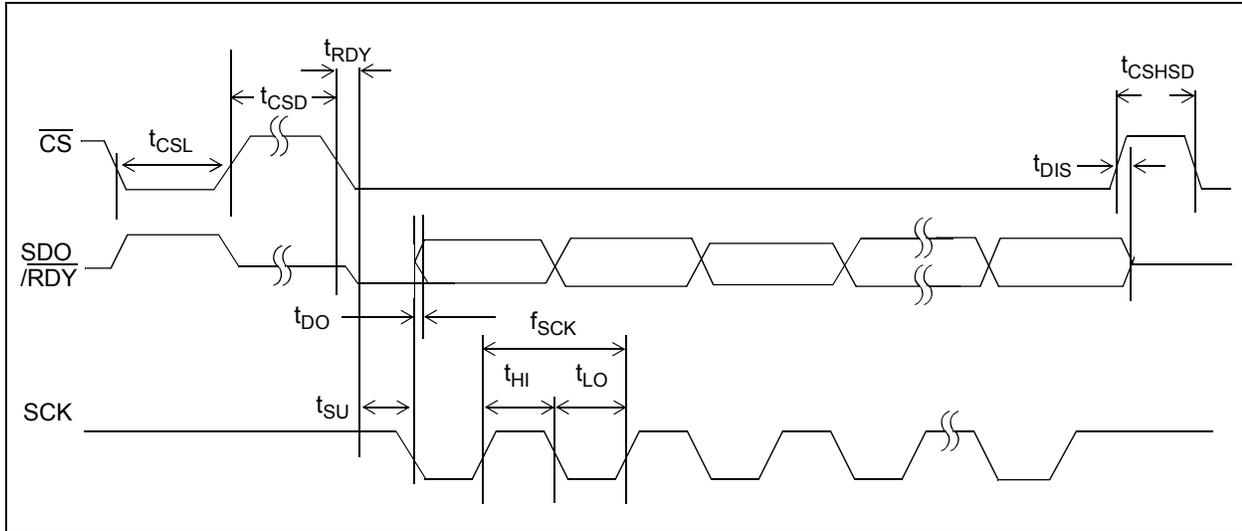
**FIGURE 1-1:** Serial Timing.
