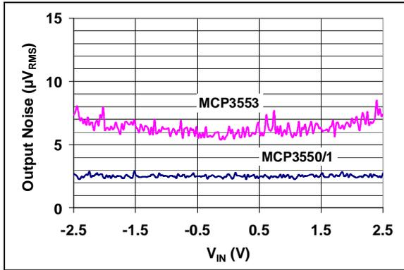
**FIGURE 2-7:** Output Noise vs. Input Voltage ( $V_{DD} = 5.0\text{V}$ ).
