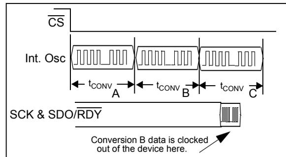
**FIGURE 5-5:** Most Current Continuous Conversion Mode Data.
