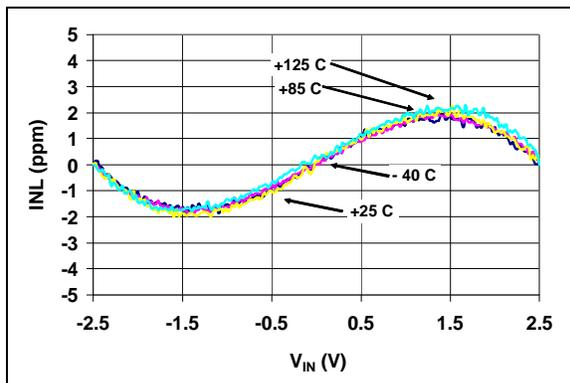
**FIGURE 2-2:** INL Error vs. Input Voltage ( $V_{DD} = 5.0\text{V}$ ).
