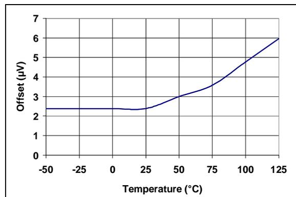
**FIGURE 2-12:** Offset Error vs. Temperature ( $V_{REF} = 5.0\text{V}$ ).
