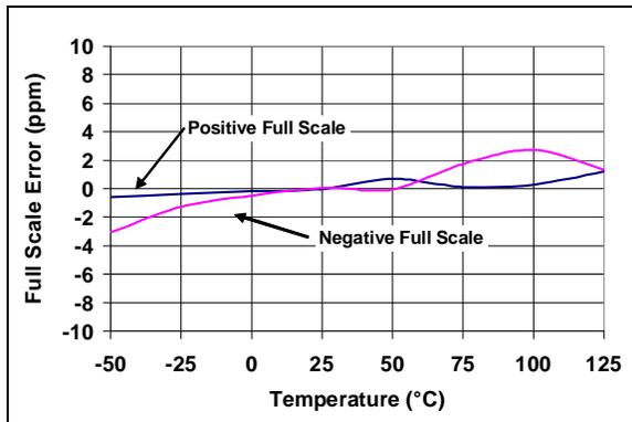
**FIGURE 2-15:** Full Scale Error vs. Temperature ( $V_{REF} = 5.0\text{V}$ ).
