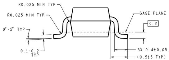
DIMENSIONS ARE IN MILLIMETERS
