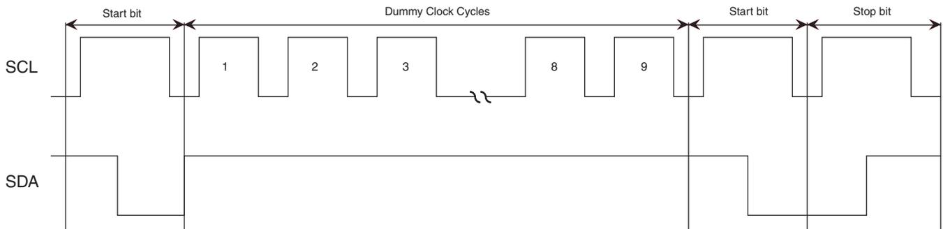
**Figure 4-2. Bus Timing (SCL: Serial Clock, SDA: Serial Data I/O<sup>®</sup>)**
