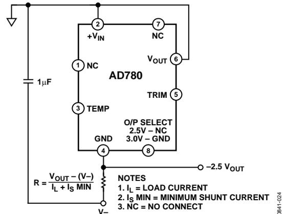
Figure 24. Negative (-2.5 V Shunt Mode Reference)
