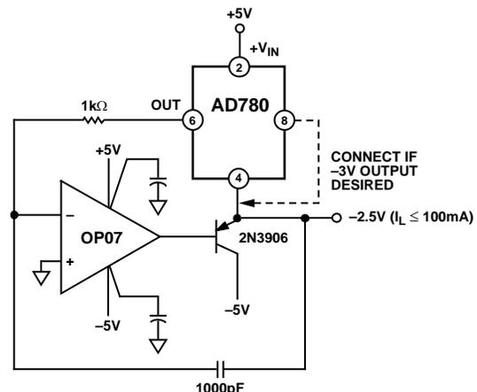
Figure 25. -2.5 V High Load Current Reference
