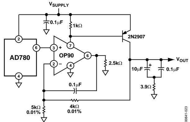
Figure 23. 4.5 V Reference from a Single 5 V Supply
