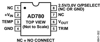
Figure 2. Pin Configuration, 8-Lead PDIP and SOIC Packages
